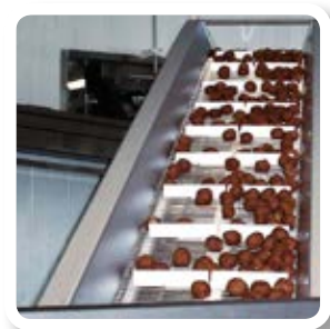
Rod network belt with POM studs in operation (inclined conveying of meat balls)
