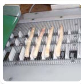
Rod network belt with individual POM studs in operation (washing and cutting machine for asparagus)
